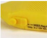
**Activating:** First remove the protective cover and press switch to activate the tool. The melting knife heats up very quickly. **RISK OF BURNING!** (Cool down period 1 minute). As soon as the melting knife is heated, the filling material can be liquefied.
