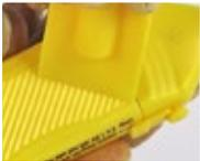
**Cleaning melter:** Use the cleaning comb to clean the planer grooves. To clean melting knife, simply wipe with a cloth after use.
