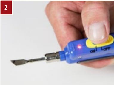
**Safety Instructions for Battery Melter:** Always store melter with cap fitted and ensure ON/OFF switch is set to OFF position. Tip becomes hot during operation. Never bring the tool into contact with water. After operation, allow tip to cool down before storage. Always turn off melter after operation, while pushing the switch into the OFF position.
